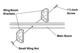
5. Insert the top and bottom wing booms into the wing boom brackets. Secure them with the four supplied 11/4-inch screws and small wing nuts, as shown.
